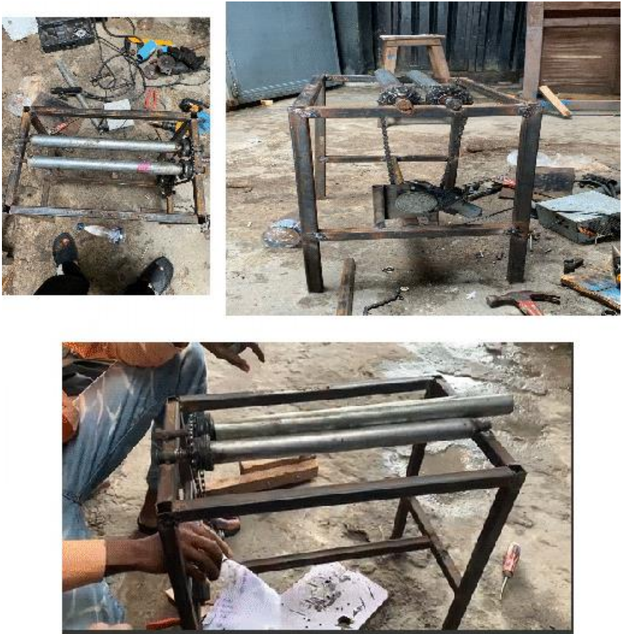
Figure 3: Fabrication of the Sheet Metal Roller
