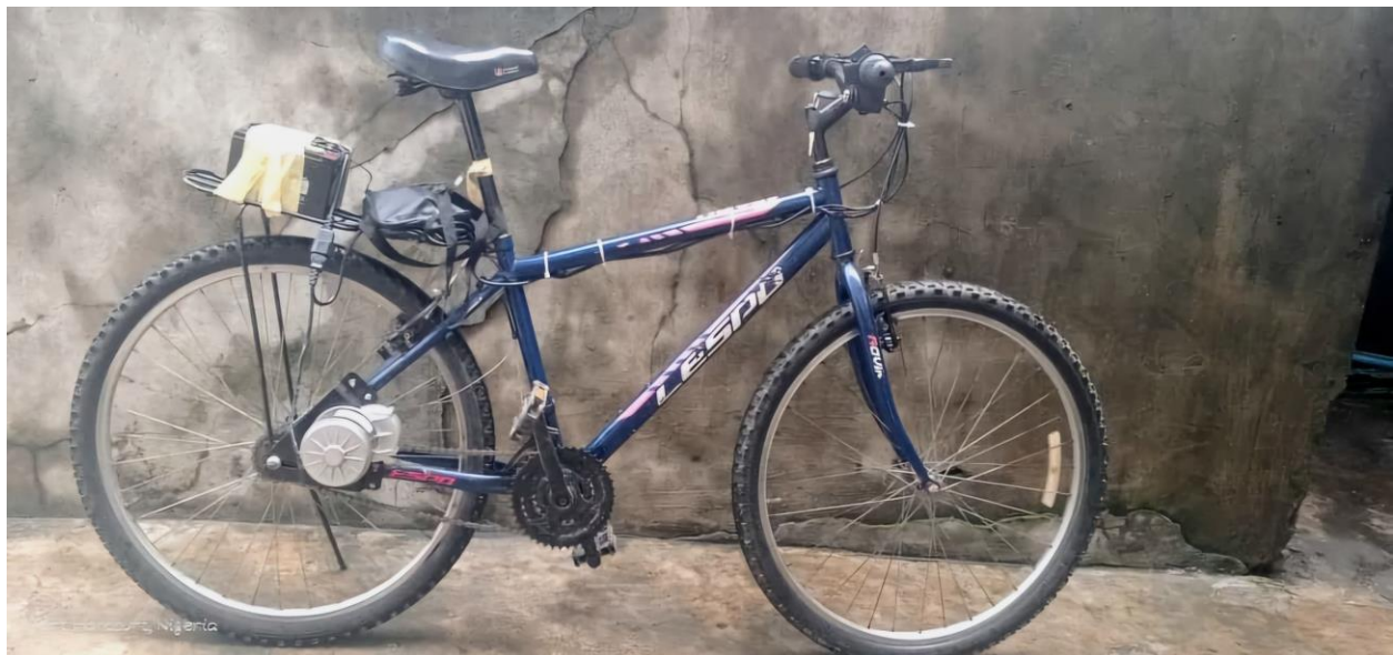
Figure 3: Pictorial view of the retrofitted electric bicycle.
