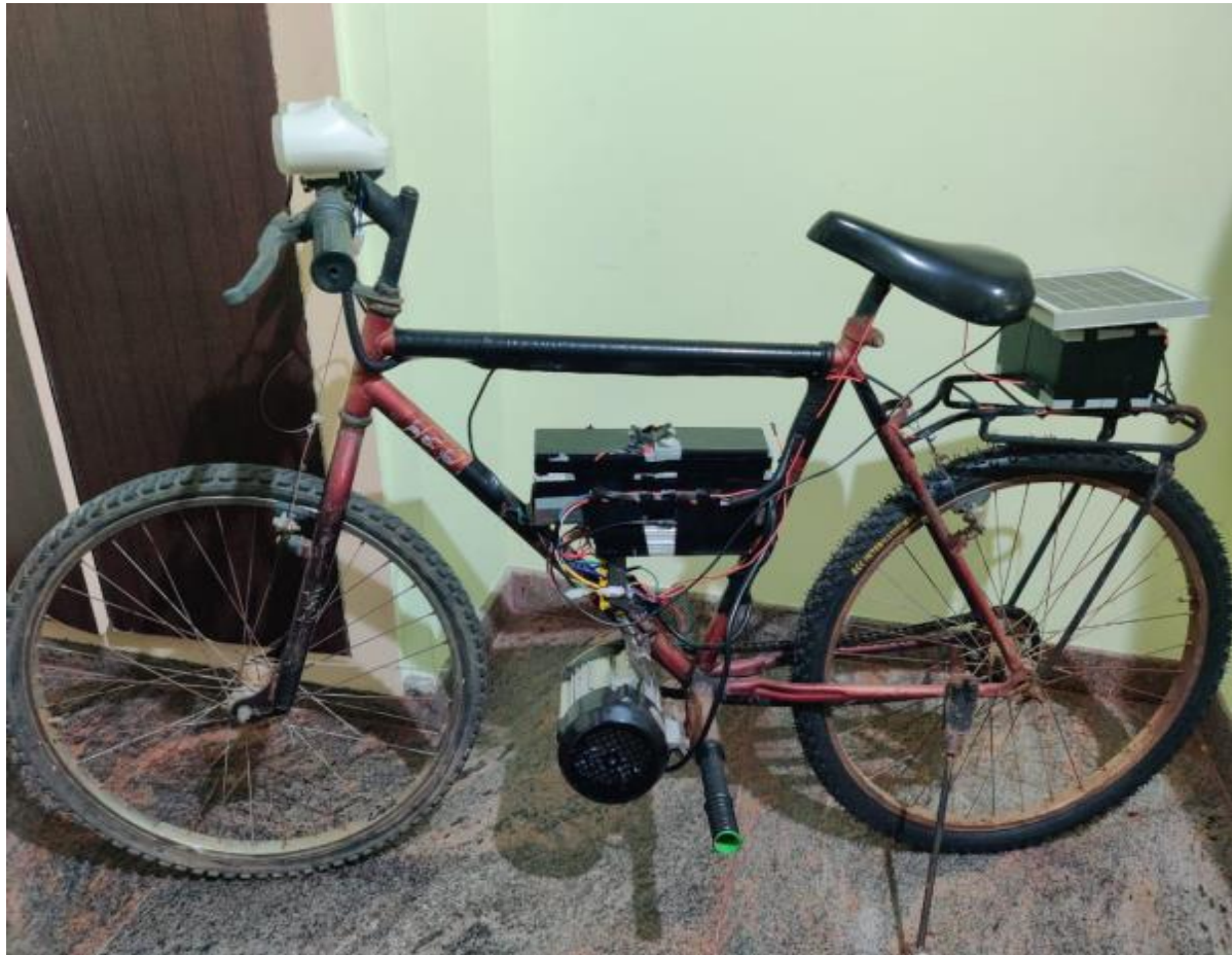
Figure 6: A solar-powered electric bicycle with a dynamo (AlSabah et al., 2024).
