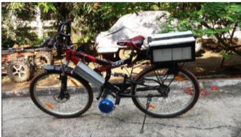
Figure 1: A conventional bicycle with electrical components mounted on it (Bansal et al., 2020).
